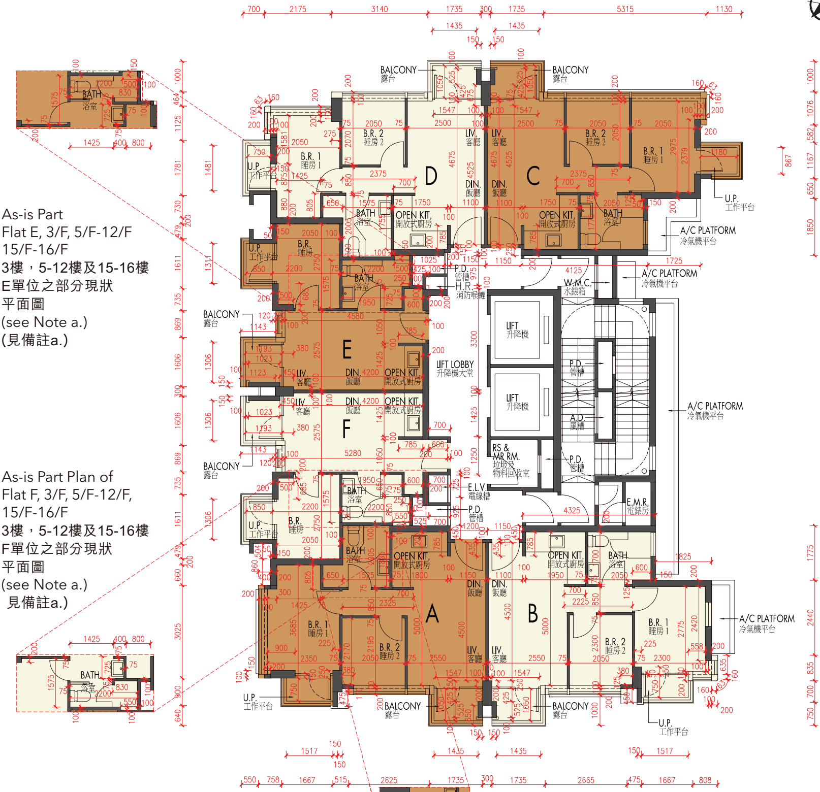
As-is Part Plan of Flat A, 16/F Existing bathroom door has been removed and new sliding door Installed.
